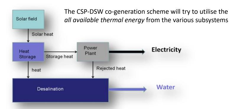
The advantages of CSP-DSW are realized only when the power and desalination cycles are integrated thermally and optimized together.
